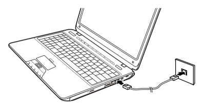
Connecting the internal modem
